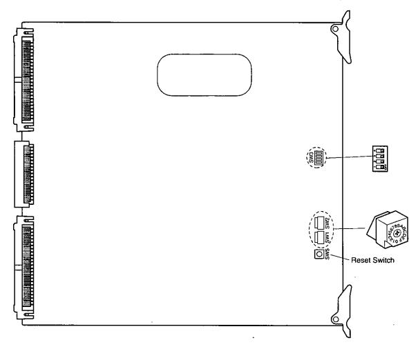
1. Set switches (SW1 and SW2) on the board to designate the On Screen Display board number as shown in the following table.
